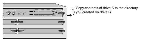
**5** After you have copied the software, replace the original NETBuilder software flash memory card in drive A with the backup copy from drive B.
